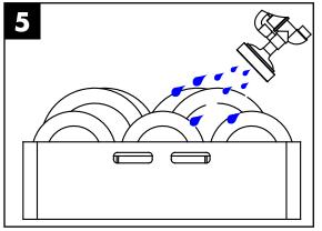
Prescrap and load wares into the machine. Wash one rack at a time.
