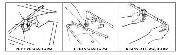
Inspect the upper and lower spray arms to ensure they are not clogged with food scraps. Otherwise, full and uniform spray pressures will not be delivered to the soiled dishes.
