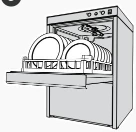
Close door, press and hold START button for 1 second and green in-cycle light will indicate the cycle has begun
