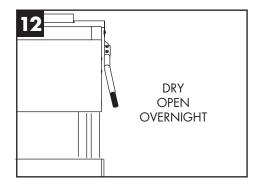
Reassemble machine and leave hood open to aid in overnight drying.
