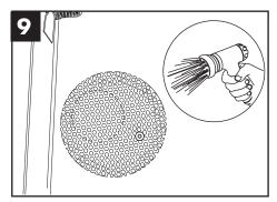
Clean the round drain screen & flush the bottom of the tank.
