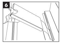
Remove the scrap screen support filler plate.
