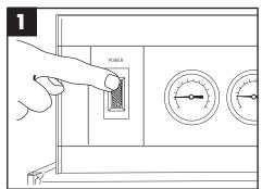
Flip ON/OFF switch to OFF position. The machine will drain automatically.
