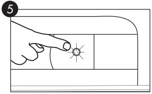
The Green In-cyle light will illuminate and the machine will start a 60 second cycle.\*
