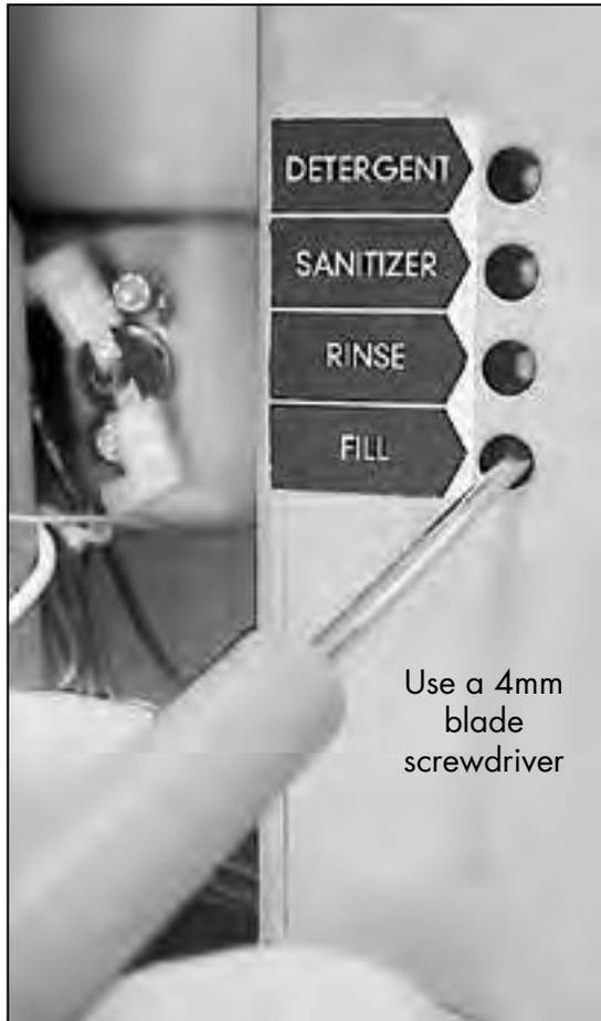
1. Adjustment screws are provided for the dispensing pumps and for the wash tank fill. They are located on the right-hand side of the dishwasher behind the lower front access panel.
