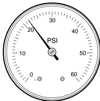
*Check the pressure gauge during the final rinse to ensure the gauge reads 20-22 psi.*
